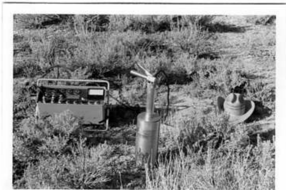
Figure 65. Neutron probe and scaler used to determine soil moisture from 30 to 150 cm depths. The vegetation corresponds to the one existing in the area around the neutron tubes in the grazed A. confertifolia stand.
