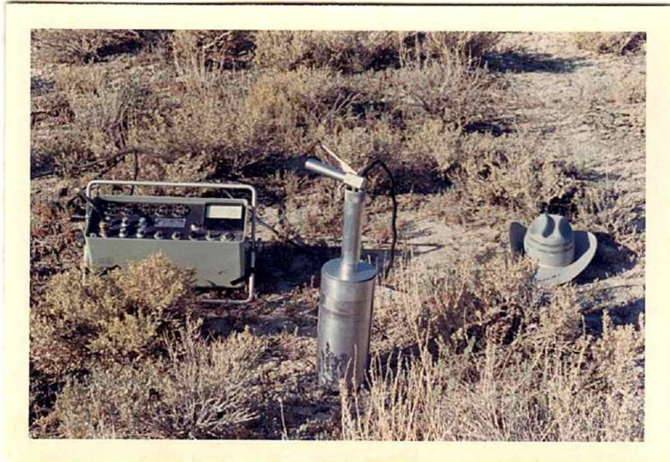
Figure 65. Neutron probe and scaler used to determine soil moisture from 30 to 150 cm depths. The vegetation corresponds to the one existing in the area around the neutron tubes in the grazed A. confertifolia stand.
